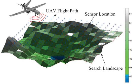
Fig. 1. Motes deployment on a sample landscape and corresponding localization with assistance of a UAV, flying on a random path and broadcasting a detection signal on the landscape.
